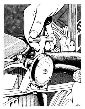
FIG. L8 BELT TENSION METER
