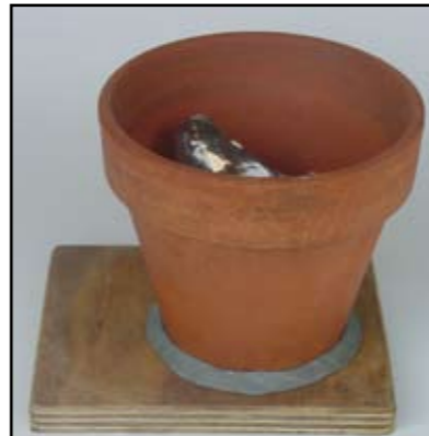
2. The container is sealed to a base and the mascot is then bolted inside the container.
