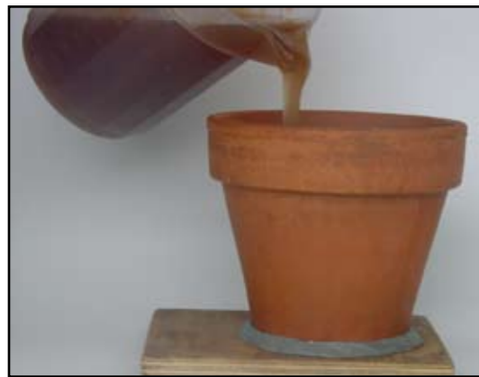
3. Heated hydrocolloid, (a liquid which becomes a flexible solid when cooled) is then poured into the container, and allowed to cool.
