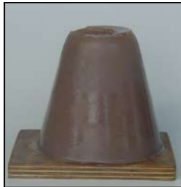
4. The mascot is unbolted from the base and the now solid hydrocolloid removed without damage because the container is tapered.
