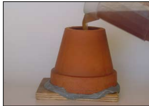
6. The sections are then re-assembled in the tapered container. They fit exactly. The container is re-sealed to the base and melted wax poured into the mould.
