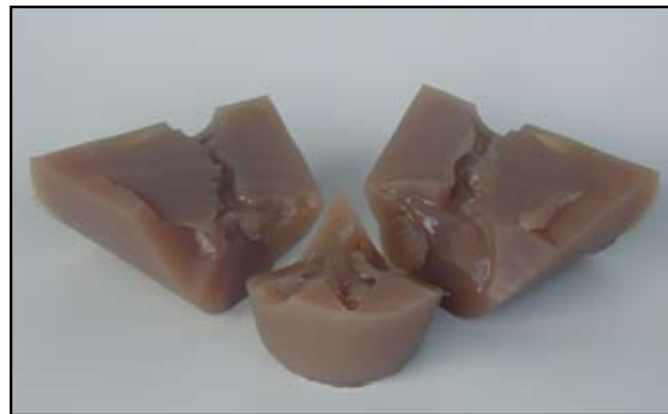
5. A narrow blade is used to make incisions in places which allow sections of the jelly to be removed from the mascot without damage.
