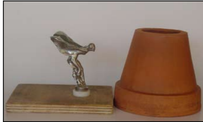
1. A sprue is attached to the bottom of the mascot. A large hole is cut in the base of a tapered container.
