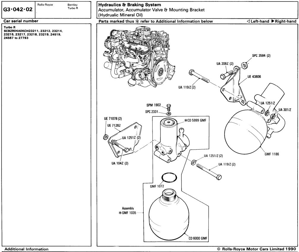
\*GMF 1035 Front Accumulator GMF 1186 Rear Accumulator \*CD 5999 GMF Front Accumulator
