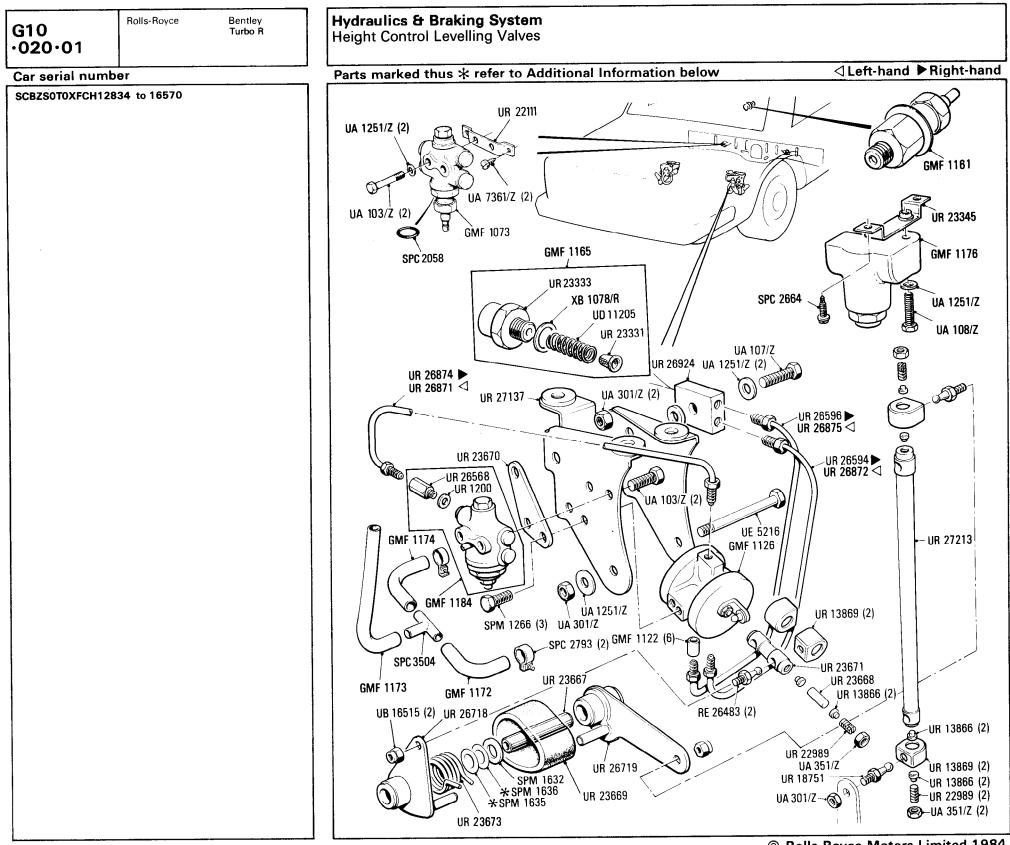
\* SPM 1636 .010 in thick SPM 1635 .004 in thick 上 as required © Rolls-Royce Motors Limited 1984
