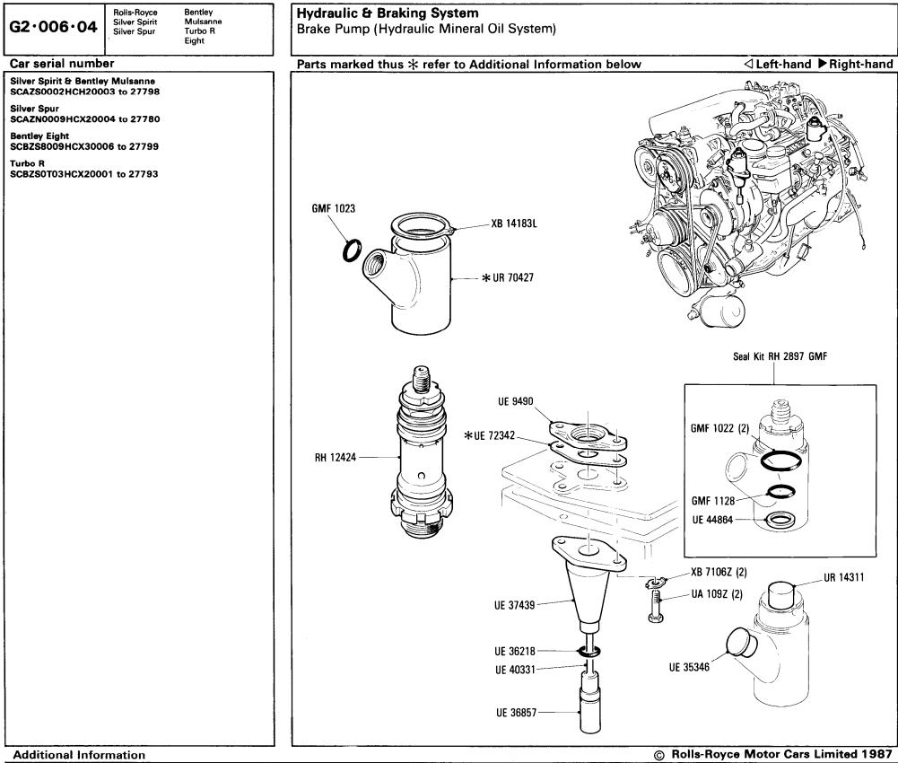
\* UE 9498 Shim .003 in as required UE 9499 Shim .007 in \* UR 70427 Front brake pump
