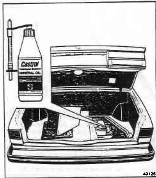
Fig. G5-3 Hydraulic system mineral oil refill bottle with special nozzle location
