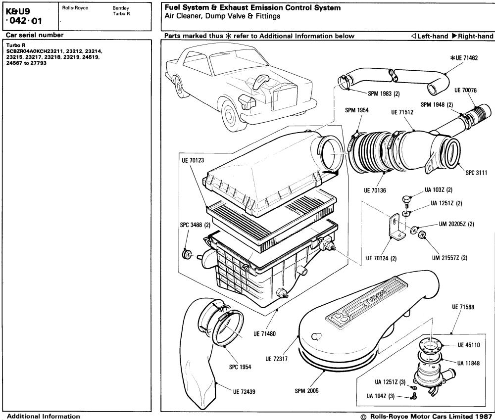
\* UE 71462 Required for car for N. America, Japan, SPM 1983 Australia, Switzerland, Austria & Sweden
