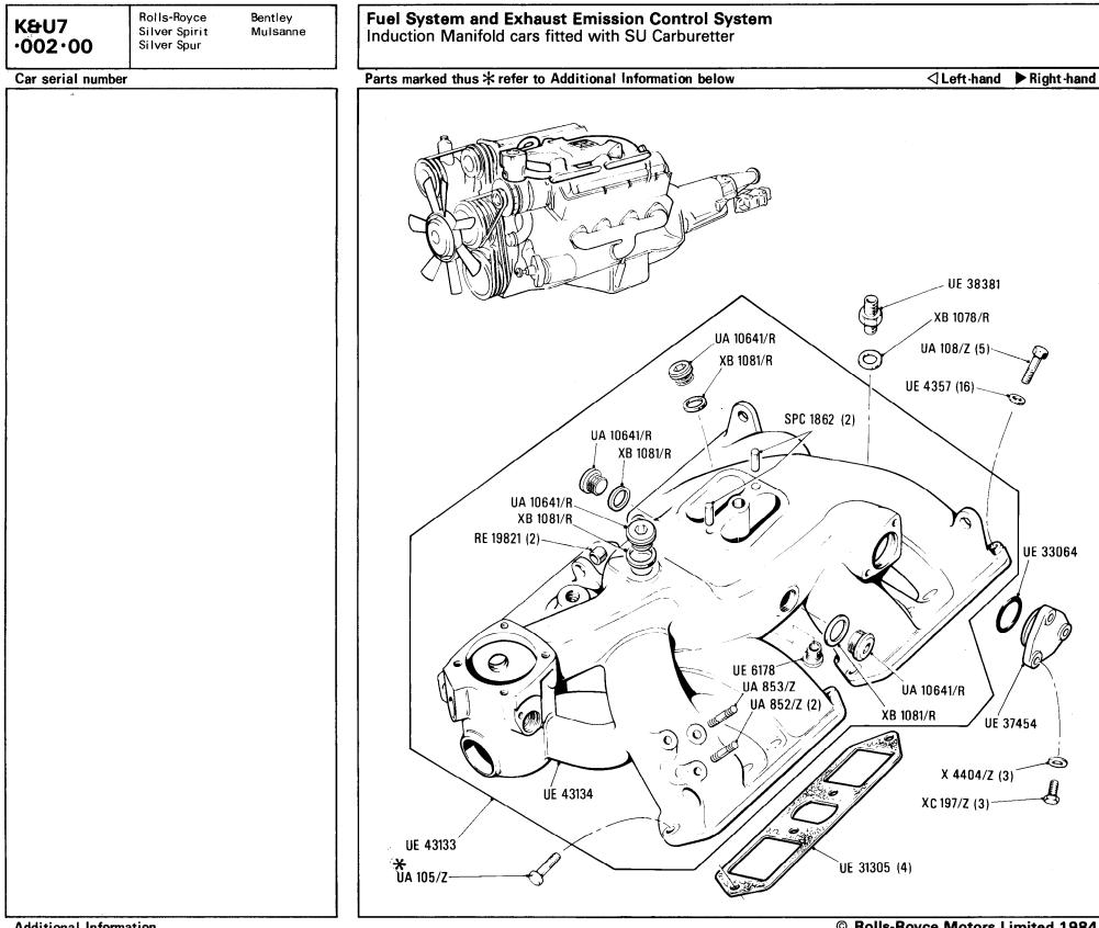
$\star$  UE 43133 Manifold with larger heater pipe aperture Introduction of larger 'O' Ring September 1981 © Rolls-Royce Motors Limited 1984
