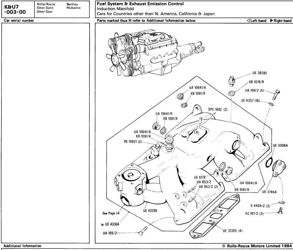
\*UE 43304 Manifold Introduction of screw in type otter switch
