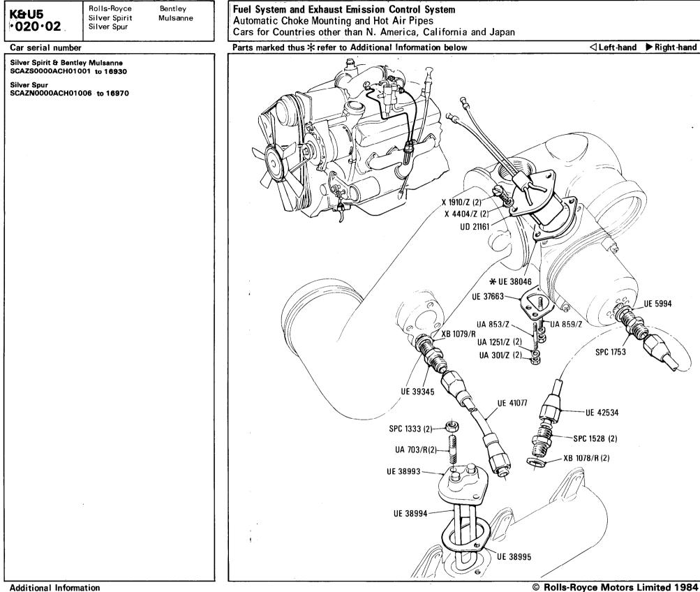
UE 38046 Adjusting Shim .002 in. UE 38047 Adjusting Shim .005 in. RD 6516 Adjusting Shim .009 in. RD 6517 Adjusting Shim .012 in.
