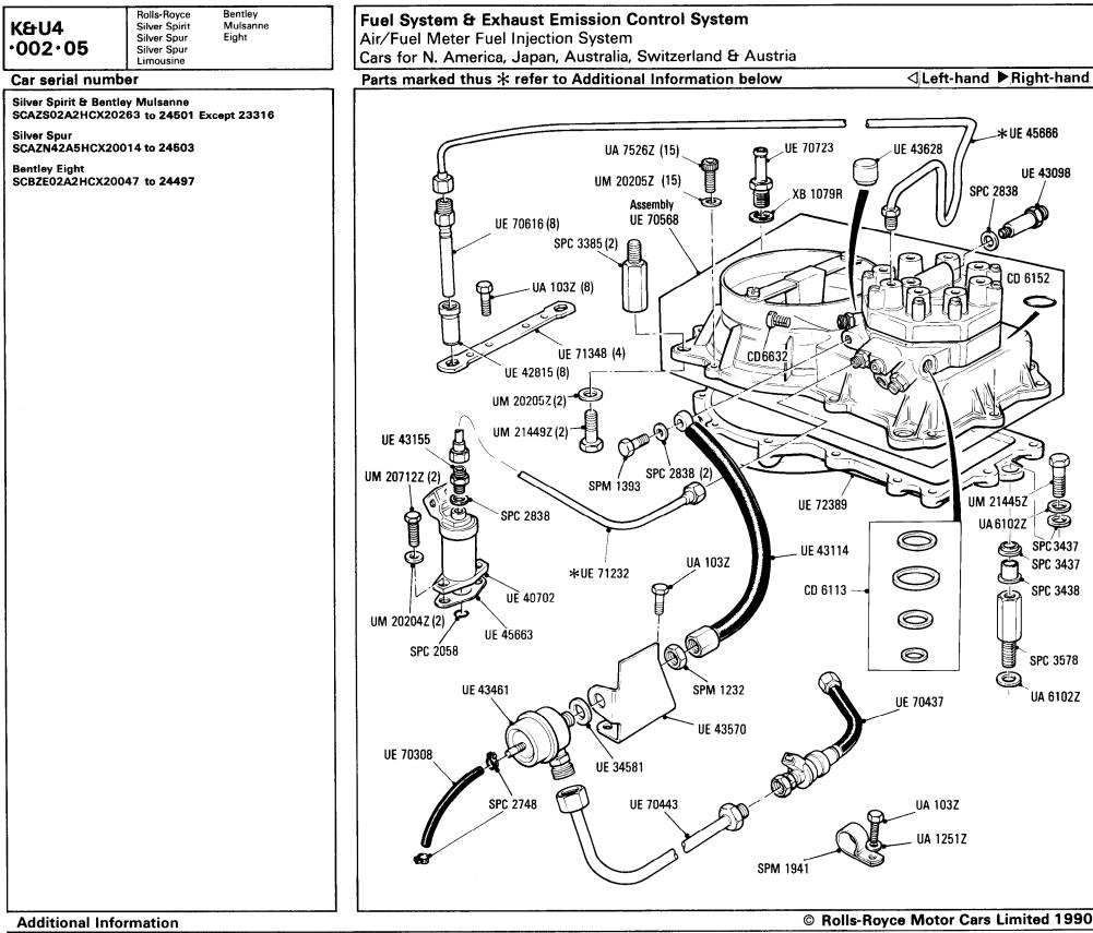
\* UE 45666 A1 Cylinder UE 45668 A2 Cylinder UE 45670 A3 Cylinder UE 45672 A4 Cylinder UE 45674 B2 Cylinder UE 45676 B2 Cylinder
