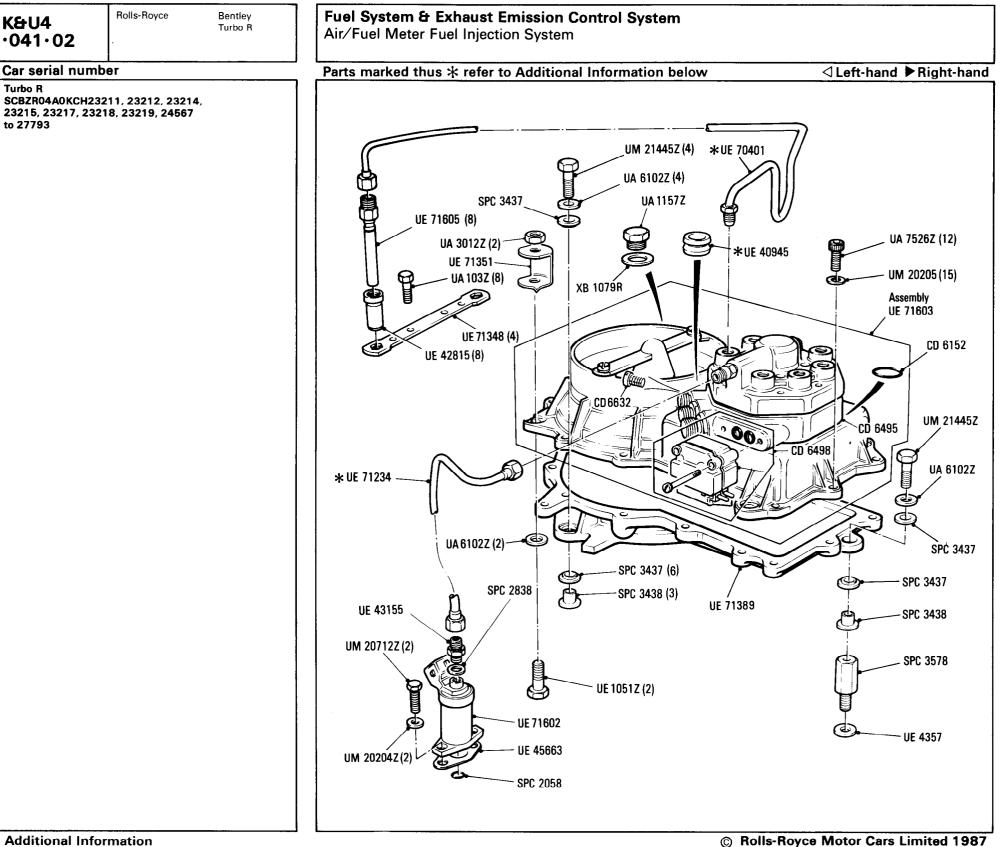
\* UE 70401 A1 Cylinder UE 45668 A2 Cylinder UE 45670 A3 Cylinder UE 45672 A4 Cylinder UE 45674 B1 Cylinder UE 45676 B2 Cylinder UE 45678 B3 Cylinder UE 45680 B4 Cylinder \* UE 71234 Pipe air meter to cold start injector \* UE 40945 Cars for countries other than N. America, Middle East and Taiwan UE 72938 Cars for N. America & Taiwan
