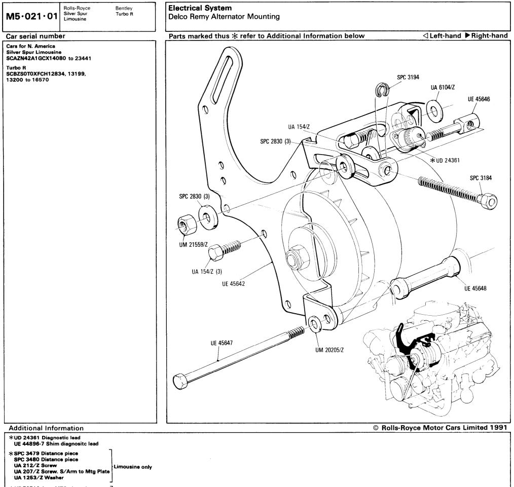
\* UE 70719 Assy MTG plate alternator UA 206/Z Screw S/arm to MTG plate 1986 Limousine only
