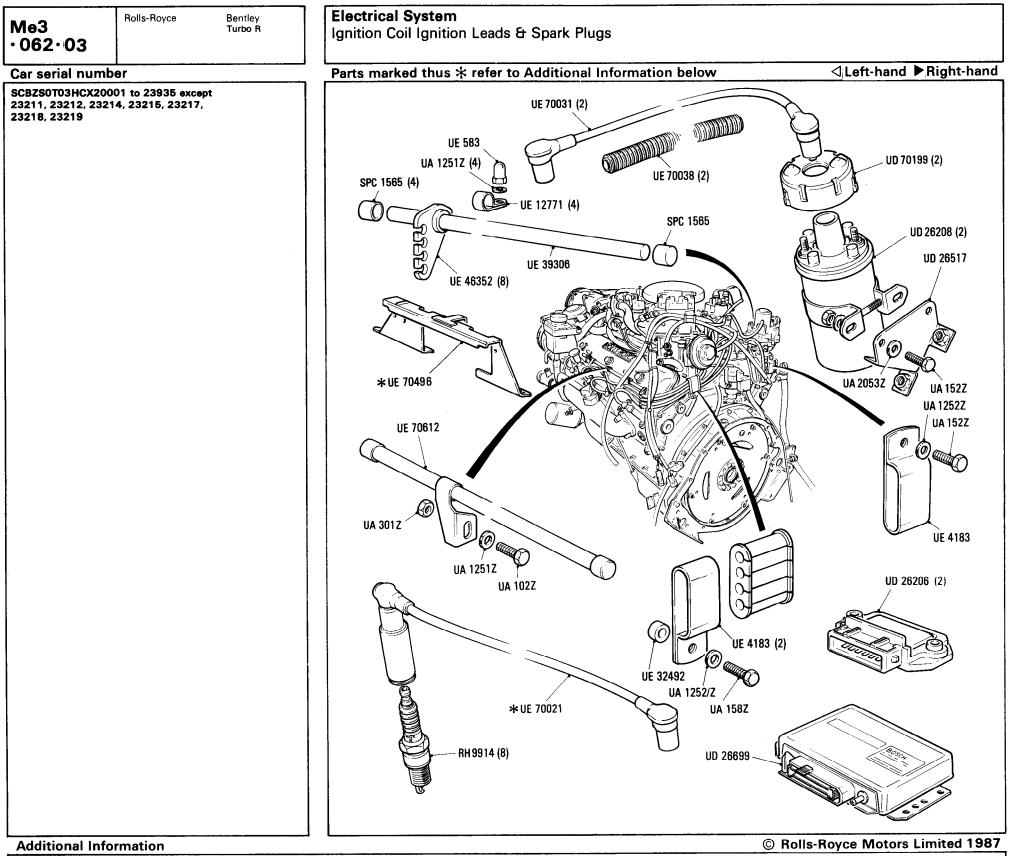
\* UE 70021 A1 Cylinder UE 70022 A2 Cylinder UE 70023 A3 Cylinder UE 70024 A4 Cylinder UE 70026 B1 Cylinder UE 70026 B2 Cylinder UE 70027 B3 Cylinder UE 70028 B4 Cylinder \* UE 70496 'B' bank
