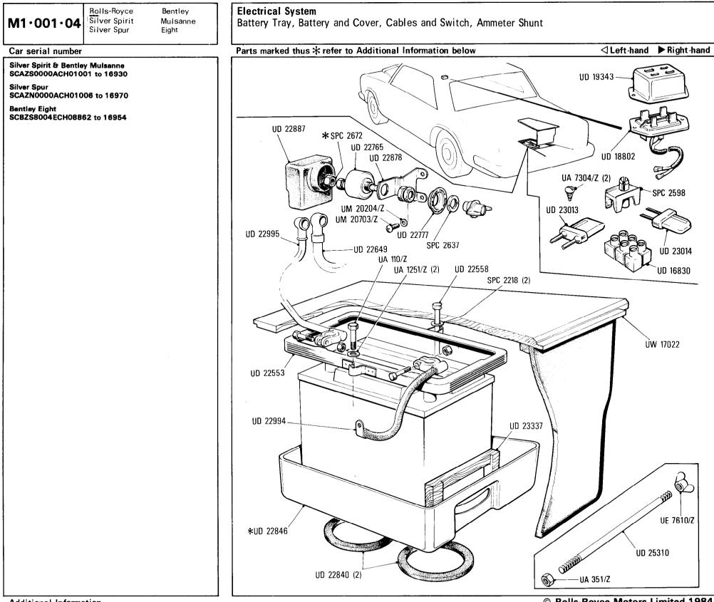
\* SPC 2672 Nylon nut \* UD 22846 Battery tray without seals UD 23910 Battery tray with seals UD 25687 Battery tray with mineral bottle holder (Early type) UD 25784 Battery tray with mineral bottle holder (Later type)
