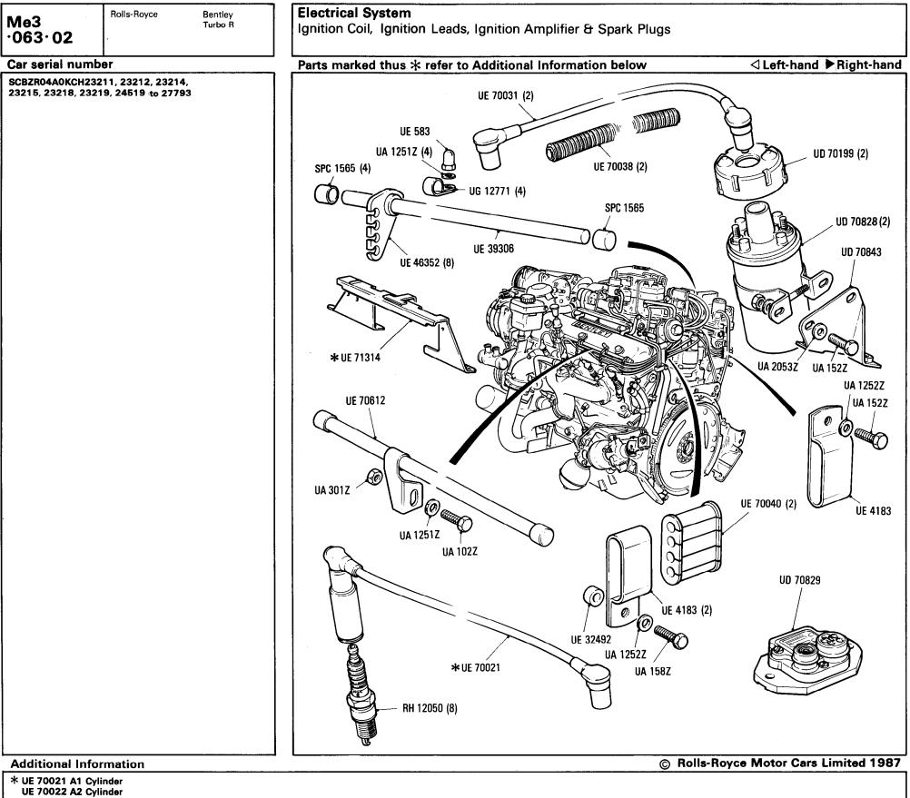
UE 70022 A2 Cylinder UE 70023 A3 Cylinder UE 70024 A4 Cylinder UE 70026 B1 Cylinder UE 70026 B2 Cylinder UE 70027 B3 Cylinder UE 70028 B4 Cylinder \* UE 71314 'B' Bank UE 71313 'A' Bank
