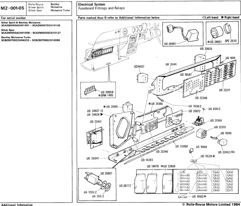
\*UD 24551 Direction Indicator flasher UD 24552 Hazard warning flasher \*UD 19102 - 20 amp fuse \*UD 11539 - 10 amp fuse \*UD 4896 - Radio fuse 5 amp \* UD 35186
