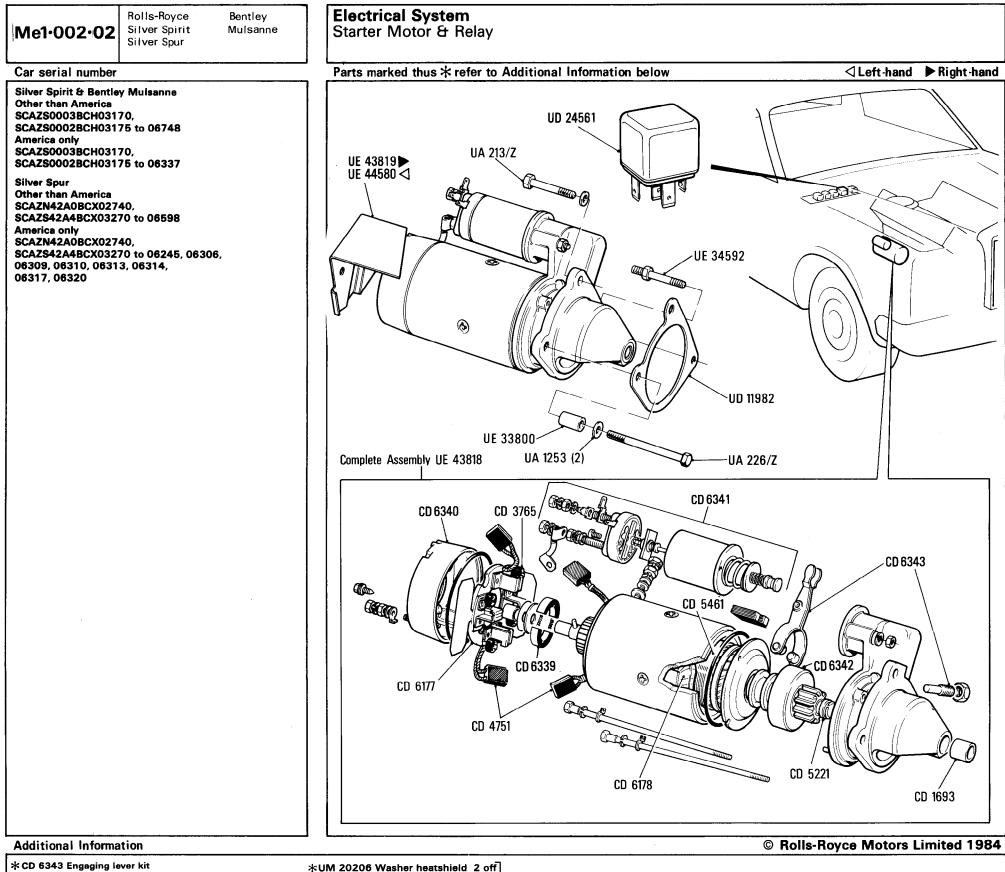
\*CD 1693 Bush kit \*CD 6182 Seal kit \*CD 6191 Sundry parts kit \*CD 5221 Retention kit \*CD 6339 Brake kit
