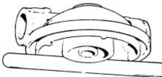
Fig.2 Inner Sealing Face Proud of Outer Lip.
