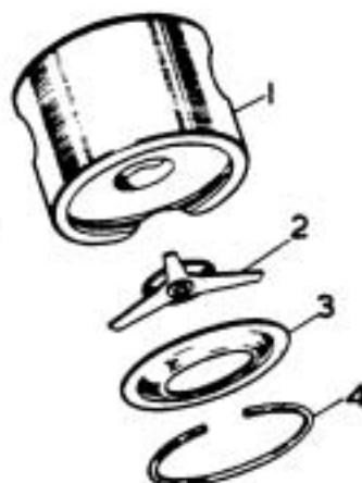
SHOCK DAMPER PISTON AND REPLENISHING VALVE.
