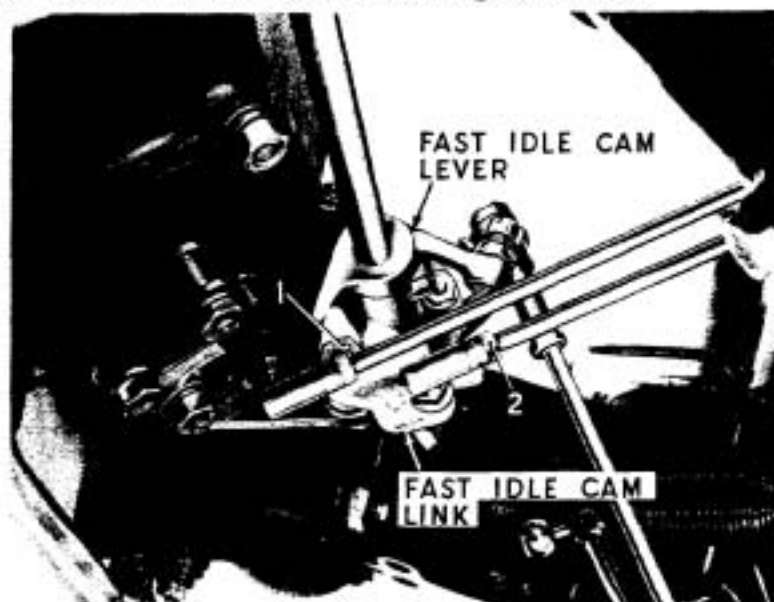
FIG. 4. THE NEW FAST IDLE CAM LEVER AND LINK.
