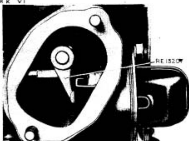
LEVER & MAGNET COIL YOKE FACES MUST BE PARALLEL ONE TO ANOTHER WHEN IN POSITION GAP BETWEEN LEVER & YOKE FACES TO BE ADJUSTED TO .004/ .006" BY USE OF SHIM WASHERS RE 17043/5
