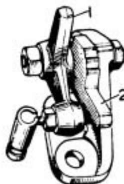
1. Fast Idle Cam Link. 2. Fast Idle Cam.
