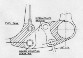
MODIFICATION TO THE FUEL TANK MOUNTING STRAP INTERMEDIATE BRACKET.
