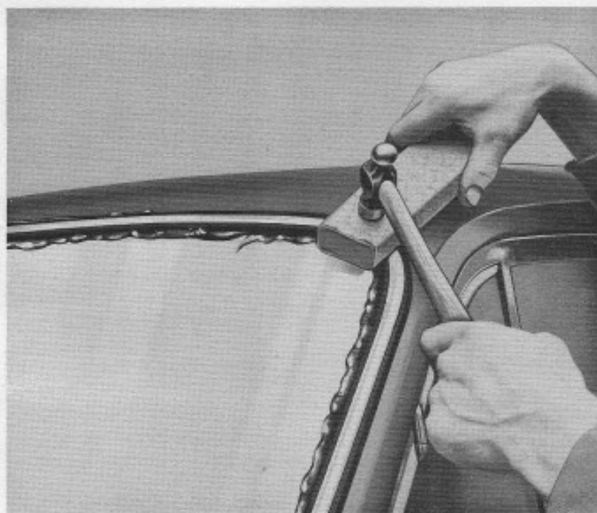
Fig. 4. Chrome finisher being adjusted after Secomastic has been applied.
