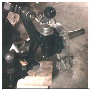
The last of the drum brakes built by the Factory. Unlike models previous to the S series and most other cars the brake shoes were mounted on a very stout plate which was bolted to the stub axle. The backing plate merely kept the dirt out.
