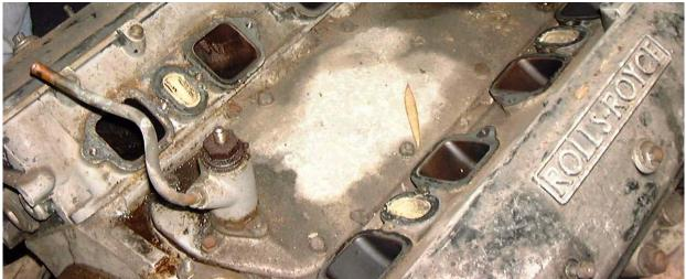
And here we have the rear of the two hydraulic pumps that often clatter away hidden among the tentacles of the inlet manifolds. To remove these pumps requires a serrated tube spanner one of which I had. Now I don't have it. Has anyone got one I can copy? The serration on the pump can just be seen near its base and access is simple once you remove the pipe, the circlip and the cover!
