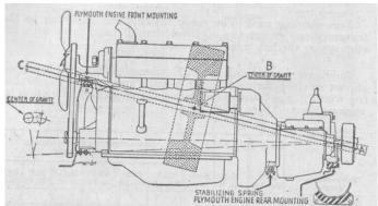
This approach was used on all cars until the advent of the 'S' series which used the fairly conventional two lower engine mounts forward and a very dinky little rubber mount at the rear of the gearbox. The V 8 engine reversed that scheme and went for one mount forward and two behind with the gearbox hanging out in limbo!
