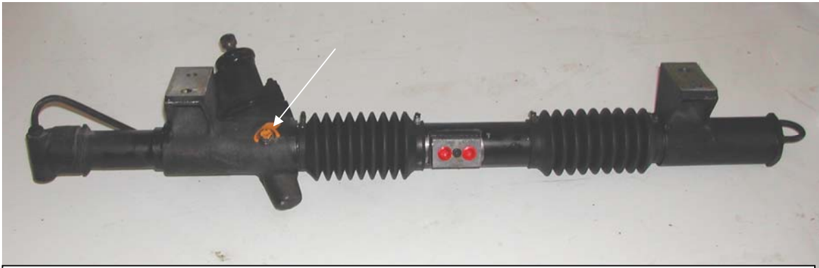
The re-booted rack – note the mounting pedestals. The screwed plug (arrowed) is removed and a drill inserted to lock the rack centrally when lining up the steering wheel on assembly.
