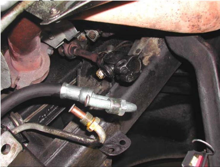
The delivery and return pipes disconnected.
