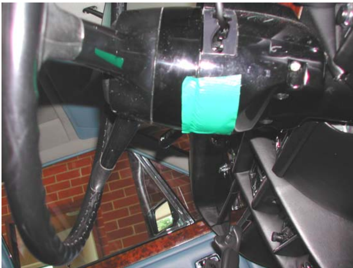
If you don't have an assistant this is one way of holding the wheel centrally while you replace the rack – some good old masking tape.
