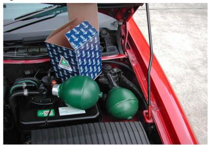
Doug's Spirit. Dimensionally they were identical as were the charged pressures. Apparently the spheres differ throughout the Citröen by the use of restrictors in the neck of the unit which are swaged in. The other difference is that the Citröen units are a third of the cost of the RR items! And the enthusiasts re-charge them!!
