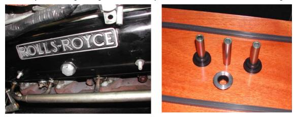
bolts on a 1985 Spirit. Some little time ago a neoprene type gasket was introduced which overcomes the shrinkage problem and provides an excellent seal. The leakage around the securing bolts was cured by fitting flat washers under the mounting bolts which have neoprene faces bonded to them. Owners of earlier cars will notice the larger blind bolts securing the cover on the Spirit. Tubular spacers over the studs prevent the cover from being over tightened.
