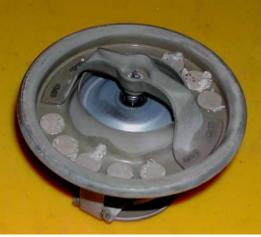
the Shadows and Spirits, it is 88°C. This is the opening temperature. Full opening is usually between 99° and 102°C. The water doesn't boil because it is under pressure (remember Boyle's Law?) The base of the modern thermostat moves downward as it opens shutting off the bypass outlet beneath it.
