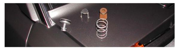
Neat paper filters have been fitted to all Shadows and Spirits and not infrequently tired mechanics have discarded them on the basis that the under floor primary filter will do all that is necessary. They are a standard commodity and should be available from your friendly local carburetter shop. Don't forget to replace the 'O' ring. The plug is extracted by a standard 7/16' AF bolt.
