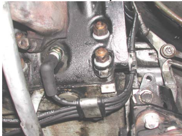
The lowest clamp for the leads on the 'B' bank
