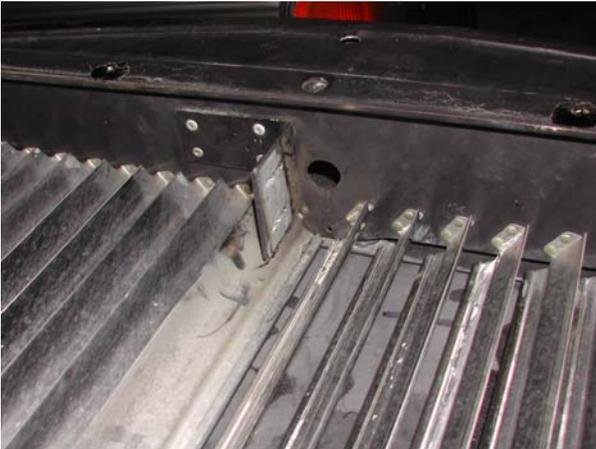
So you want to startle people fiddling with the lady? Fit a mascot alarm. There are plenty of home made variants on this modification but here is how the factory did it on a Silver Spirit. Here is a stout aluminium bracket mounted on the header tank. The foot of the mascot which is spring loaded sits just above the whole seen in the picture. The switch which is mounted within slots in the bracket pokes up the hole until the internal contacts
