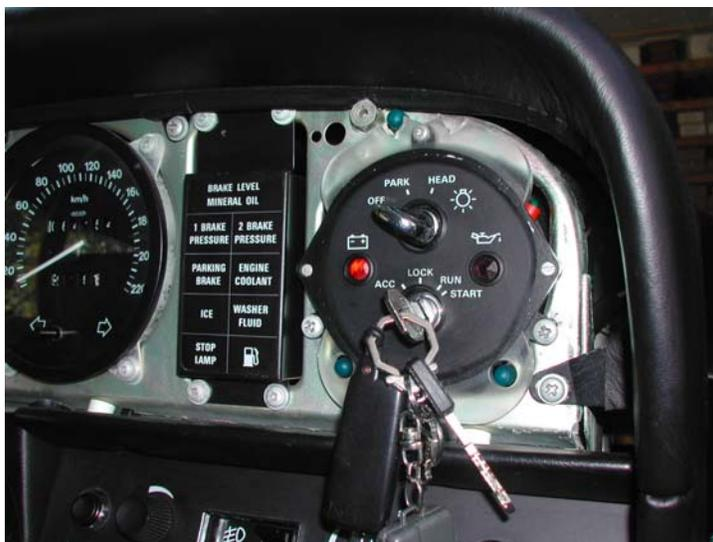
Restorers know of the difficulty in bringing switch boxes back to life after having been gouged by swinging keys and drunken drivers. From the Shadow II the factory screwed a face to the box which is based on 3/16" plastic sheet. Ingenious, as it allows a whole variety of languages and symbols insisted upon by the various customers. It also allows peripheral lighting as can be seen in the picture.
