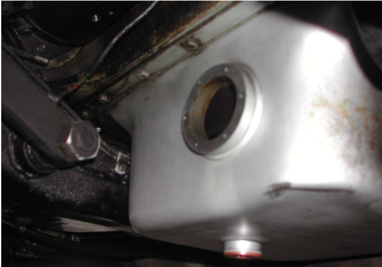
Looking aft on a 1975 Silver Shadow. This is the hole left after the sump level unit is removed. The unit is mounted on a welded-in ring seen here clearly and sometimes there is a leak between the ring and the main sump. That involves removing the sump and some clever braising and re-plating.
