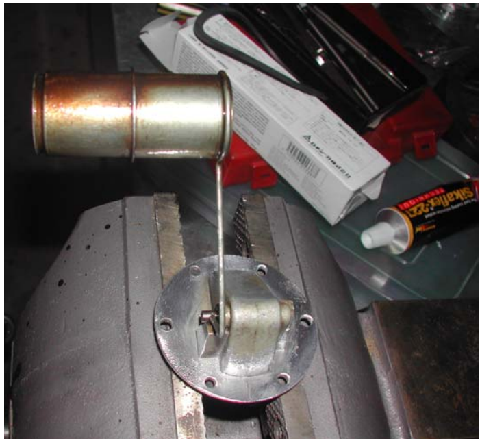
The business end of the unit. The float can puncture as any other and the quickest way to check this is to immerse it in boiling water. A string of air bubbles will prove a hole and its location. A dab of solder after draining the float fixes it.
