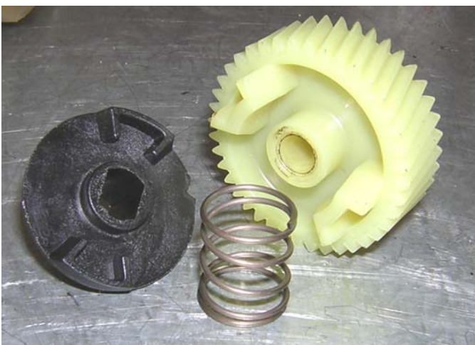
One of the clutches. Note that the gears spin freely on their shafts but the clutch is keyed to the shaft. When the solenoid pushes the clutch into the gear the latter turns the clutch which in turn, turns the shaft which in turn, turns the Bowden cable!
