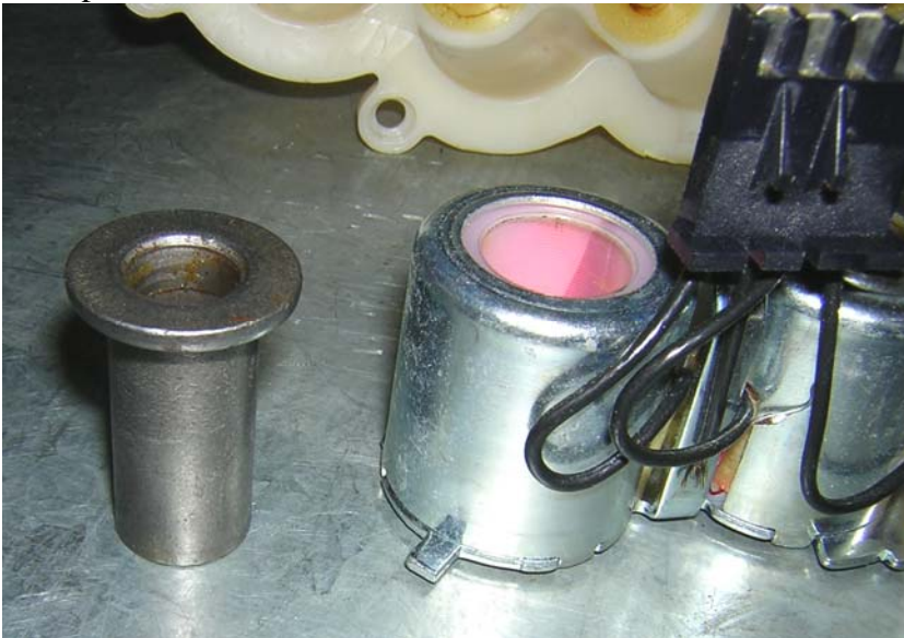
One of the solenoids and armature. Powering the unit pushes the armature left out of the solenoid and lifts the clutch against a return spring to engage the respective gear.
