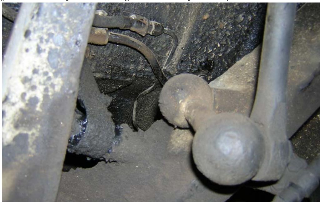
The filthy things on the left is the retaining strap which should be kept well greased
