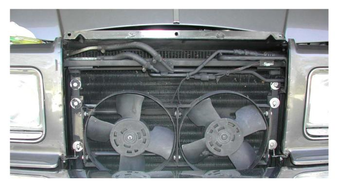
And while on hoses don't forget the little darlings behind the grille. Seen here on an '85 Spirit they connect the low pressure side of the power steering system through a variety of heat exchanger to try and keep the oil at a reasonable temperature. They are not eternal and usually dribble a lot which is difficult to pick up. But when they eventually blow the result is quite spectacular with jets of oil squirting out of the front of the grill. It is difficult to ignore at this stage.
