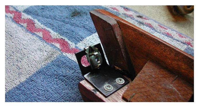
The above is the front end of one of the rails. The captive nut is a metal thread and not infrequently you will find vandals have been there and inserted self tappers. The assembly is the one into which the end screws (5) under the door seals screw.
