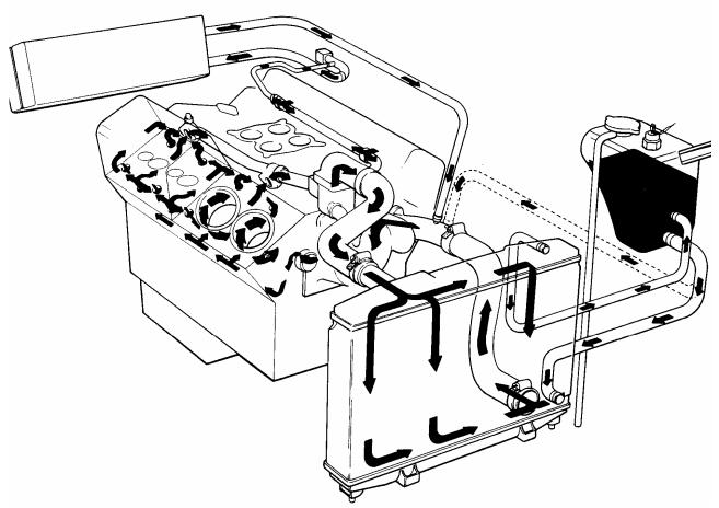
Here the overflow bottle becomes part of the header tank in effect and is itself pressurised. Note that the top of the radiator no longer has any filer cap. In the event of a major loss of coolant the bottle would immediately empty, the sensors would be exposed and the alarm would light on the dashboard. It is probably not practical to upgrade the old system but one solution seems to be to fit the audible alarms detailed in the last Topics. Silver Shadows of course don't have this problem.
