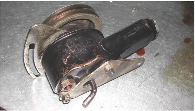
The above is a later pump used by many car makers and replaces the old Hoburn Eaton pump used on the Silver Clouds. The only repairs (apart from panel beating) these pumps seem to need is seal replacement and with age the replacement of the main shaft bearing which being basically white metal crystalises with age.
