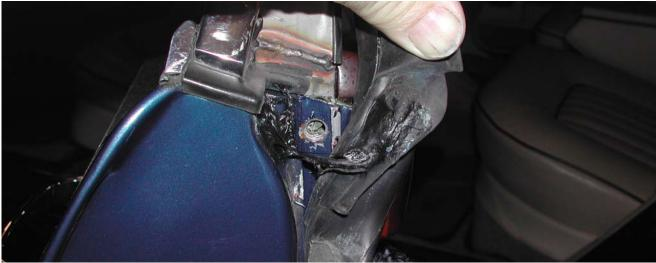
One of the elusive end screws. When you deliver the rails to the finisher you may choose to remove all the hardware or leave it to him. Note however that the window side seal attached to the glass side of the waist rail requires both gluing and stapling.
