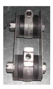
Above is a happier assembly with new washers and springs as well as new carden joints and a centre bearing. Recently I had a nice ride in a dear old 20/25 HP. The owner was reluctant to exceed 55 MPH at which speed there was a very intrusive high speed vibration. The source had to be the tail shaft and this was proved when the car was put in neutral and allowed to coast. The vibration stayed. The cause was probably worn universals and general unbalance.
