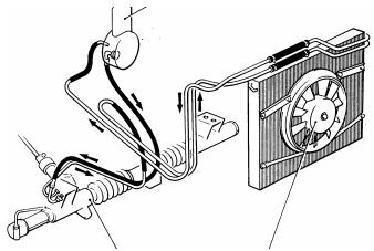
This schematic applies to the Silver Shadow II and the Spirit. The oft forgotten small hoses behind the grill are clearly shown and which should be inspected regularly for leakage.
