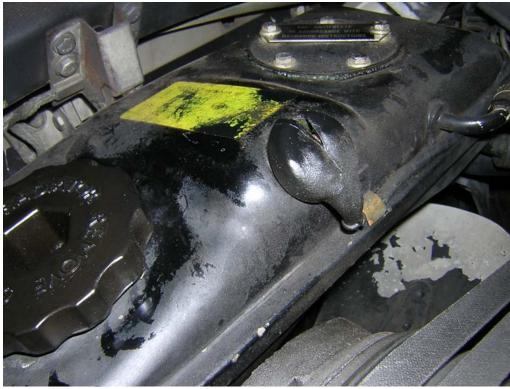
There are three things staring at you here. The filler cap, the cover of the level sensor and the steam valve cover.
