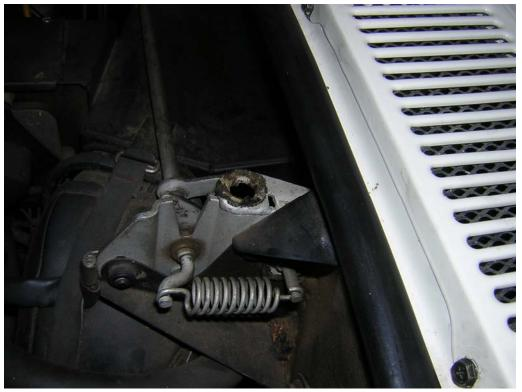
None of my readers would be guilty of this, a missing bonnet cushion – see the dirty hole in the centre and no filter on the air intake for the air conditioning. Both items are used on both Shadows and the Spirits and their derivatives. Both are important. The bonnet cushion is the only positive locater for the panel. If it is not there the thing can get damaged if slammed but more likely the sideways movement of the
