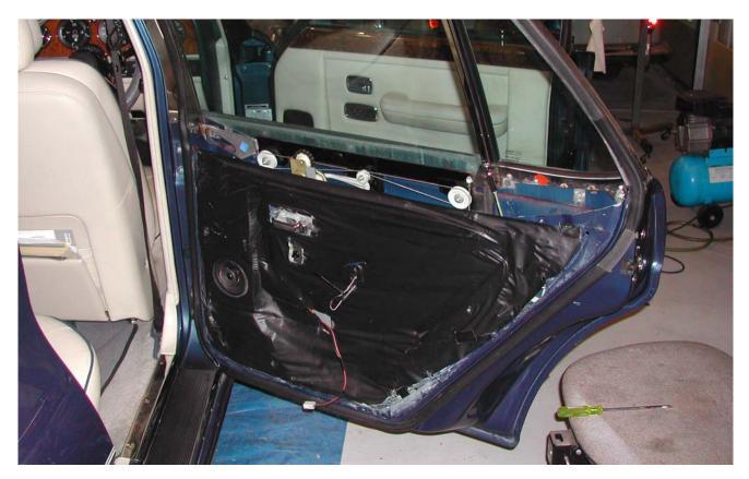
If the fume seal or plastic liner is missing or badly torn get a sheet of builders' plastic and make a new one. Without it moisture that inevitably gets down into the door will damage the door liner and rot the wooden base.
