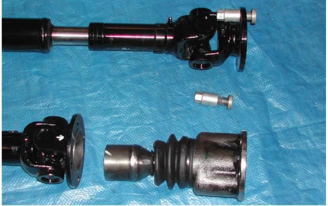
The latter of course allows the shaft to alter its length as the rear axle swings around the front
