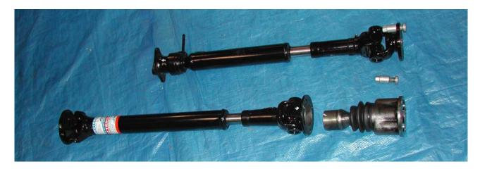
The rear shaft shown as the lower one in the two pictures posed no great problem as the universal joints are perfectly standard Hardy Spicer units as is the sliding joint at the front of the rear shaft.
