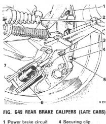
2 Master cylinder circuit bleed screw 5 Locating pin 2 Master cylinder circuit bleed screw 7 Pad adjusting
