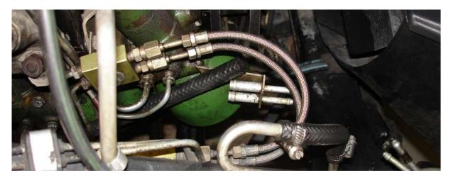
The twin pipe restrictor seen on the Silver Spur in the middle of the picture is mounted on the front of the accumulator valve. The disconnected hose is the large return pipe from the number 2 accumulator located on the side of the engine block. Using this fitting on the T2 obviously used up only one of these restrictor pipes. To the right can be seen the entry ends of the return pipes to the reservoir.
