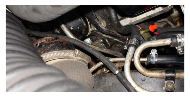
A not terribly helpful picture of the installation in the T2. The unused 'leg' of the restrictor still has its red blanking plug. The black hose beneath the red cap is the smaller end of the return pipe which is curved around and joins up with the steel chassis pipe seen immediately below it. Unlike the Spur which because of the juxtaposition of the accumulators to the body frame there was not much opportunity to run reasonable lengths of flexible pipe.
