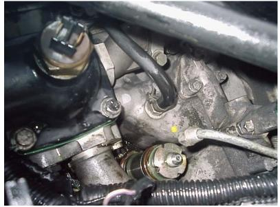
The outer casing of the front pump removed.
