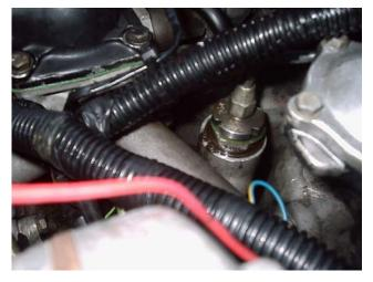
open-ended spanner in this case and 10 minutes of bad language. Then, I undid the top highpressure pipe union with a <sup>1</sup>/<sub>2</sub>" open-ender, and bingo: off came the outer housing, rather freely I may say.
