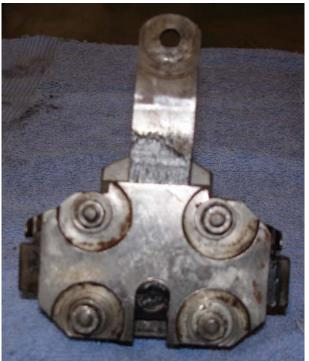
the combined hydraulic double acting piston that applies the rear brake shoes in your Cloud. If they should fail the wide rod seen protruding from the assembly, working through rollers and cams manually applies the same brake shoes.
