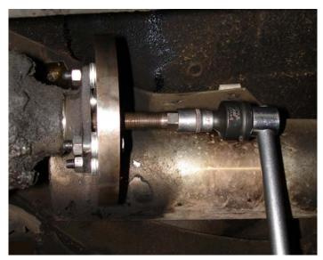
You should also go to your nearest bolt shop with one of the propeller shaft flange bolts in your greasy hand and purchase four high tensile bolts and nuts, the same diameter as the flange bolts but long enough to go through your puller and the flange leaving enough to get the whole new nut on.
