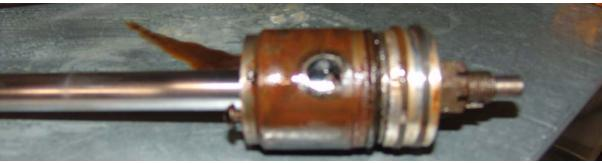
And here is the grotty plunger bearing and piston complete with rings. The large hole in the bearing receives the front feed nipple. The piston is a very simple device with very ordinary rings.
