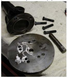
you will most certainly bend the flange and even run the risk of breaking it! Go to your local friendly fitter and turner and ask him to make up a stout disc of good steel about an inch thick with a central threaded hole. He will tell you where you can get a suitable mandrel (the high tensile pointed bolt screwed through the middle).
