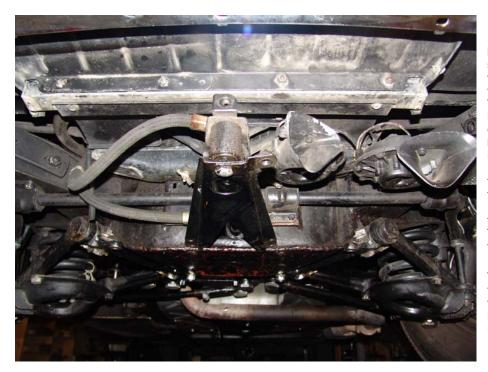
Here is the ram mounted between two substantial support plates which in turn are bolted to the front cross member. hydraulic supply hoses that feed into the cylinder at either end can be seen on the left. This is a later installation on a Phantom where the forward hose feeds into the top of the cylinder rather than the side - a feature of the earlier cars. The latter made bleeding the system more difficult.
