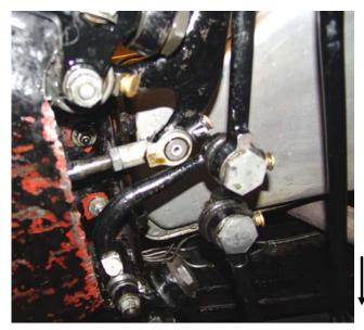
And on the other side, the plunger emerges to connect with the primary steering relay lever. This is the disconnect point for the ram. The lock nut seen on the plunger shaft is loosened after recording the number of threads exposed behind it and the shaft can then be screwed out of the swivel piece on the relay lever.
