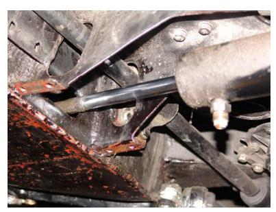
The plunger emerging from the rear of the power cylinder and passing through the front cross member. Here the lower support plate has been removed and the cylinder puled well forward. The front anti-roll bar can be seen above the plunger.
