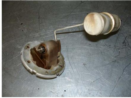
This is the float that bobs around in the sump to tell you what is the oil level. There is a new thin gasket plastic sheet supplied for the joint between the float assembly and the side of the sump which at last appears to have stopped the perpetual leak that existed has on all preceding cars. When you remove the retaining screws note that each one has a star washer and a very thick washer under the head. The thick
