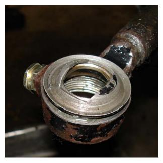
At left:- Here is the tie rod housing into which all the gubbins screws. What you don't remove is the upper bronze cup into which the ball pin is forced. This can be seen through the central hole. If this has to be replaced it requires a press to remove it.
