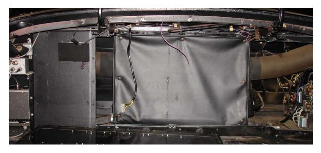
And here is the rear boot air conditioning unit. The delivery pipes seen directed to either side of the boot connect with plenums delivering cooled air to ceiling ducts and controlled ducts at either
