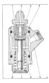
And here is the pump in section. The dark dots are the errant 'O' rings. There really is little to go wrong with these pumps other than they get clogged up through neglect.
