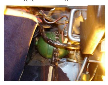
system the car will need to be standing on its wheels. Exhausting the system will let the car sink to a very low level so don't lie underneath while letting the pressure go otherwise you will probably remain there for the rest of your life! You can jack the car up and stand the rear wheels on car ramps or large blocks of wood. Post '86 cars tied both sides of the system together on the one circuit so one bleed screw will empty the lot!
