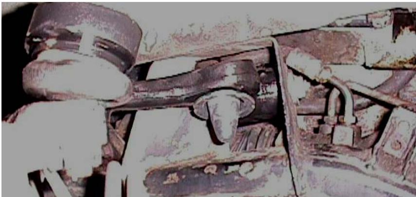
The rebound rubber. The front road spring has been removed to facilitate replacement of the shock dampers. This one is the wrong rubber. This is used on the very early non-compliant suspension. If this rubber is used the whole moulding will skew around the sub-frame and eventually allow the mounting cup to hit the frame.
