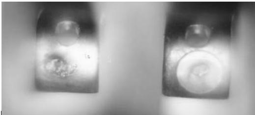
Burnt contact points - easily cleaned up with a point file.
