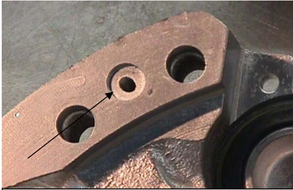
The hole (centre) connecting the hydraulic circuit between the two halves. There is a
