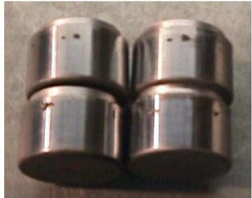
These pistons just passed muster as the corrosion pitting was outside the
