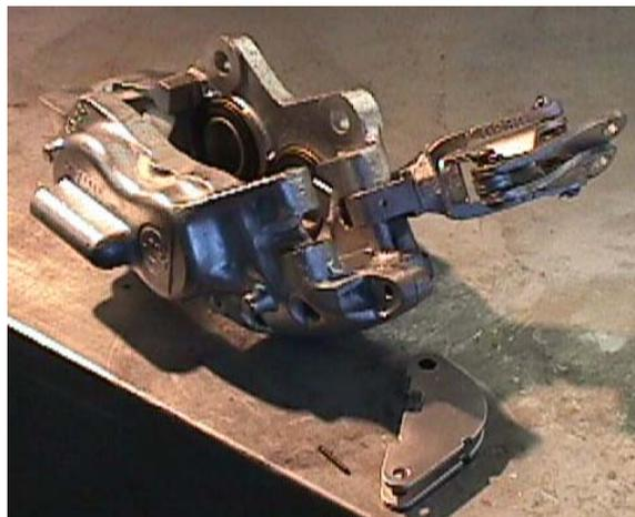
Here is a case of one of the brake levers falling off because a roll-pin has corroded
