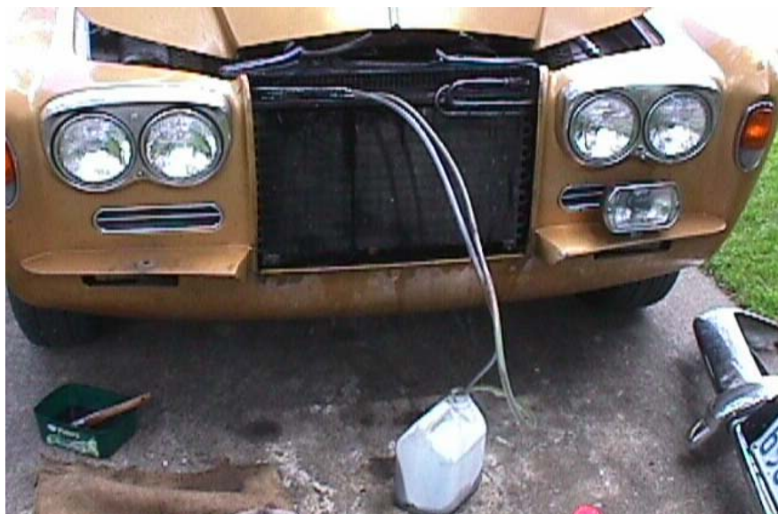
Another method of flushing the power steering
