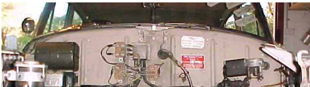
The flasher relays for the fog lights fitted to an S2. The flasher units are located above the steering column behind the dash panel
