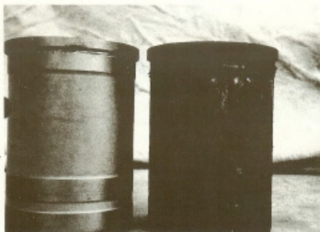
The old sleeve shows why the sleeves are often well-secured to the block. The build-up is basically aluminum corrosion.
