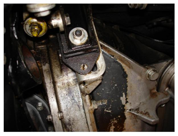
The engine on the move. The rear mounts have been disconnected allowing the whole engine to be slid rearwards exposing the rear set of bolts of the sump seen bottom left. There are still more bolts above the sub frame but more sliding forward and a little lifting allows you to get at them. The orange daubed nut at the top of the picture is the bottom end of a little shock absorber between the engine and the sub frame. Some cars had them others didn't. Why? I can't help perhaps you can!
