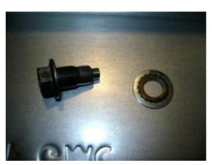
The last bastion for foreign material, a magnetic drain plug complimented by a modern day version of the doughty washer. Fortunately the latter can be used several times. This is probably the best practical feature of the later version of the transmission in that you can drain all the fluid from the main casing without drowning yourself in the stuff as with the old arrangement.
