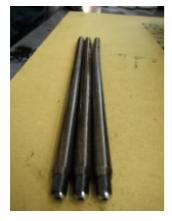
Seen here is the valiant push rod that tried to force the valve open and bent itself in the process.
