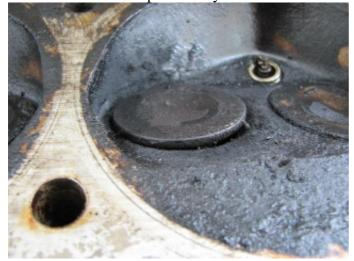
The owner of this engine was proceeding with the rest of his car at great speed when this strange miss and knocking occurred. Such things do little for the lower portion of the driver's alimentary canal! Apparently one of the exhaust valves had seized in its guide and stuck open.
