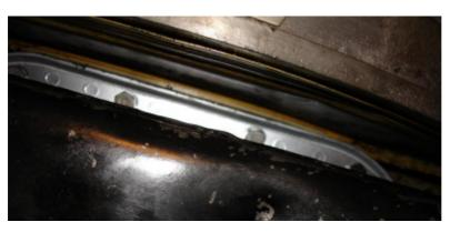
And here is why you have to slide the engine. The rear bolts holding the sump on are just that bit inaccessible to get a socket on them.
