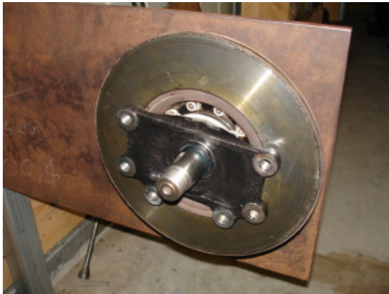
At the base of the axle there is a retainer with a felt seal squashed into it. This should be replaced and lightly greased to allow the drive shaft to be inserted. Here the shaft is waiting for the Woodruff Key to be inserted, the yoke pushed on and the nut applied to secure the assembly.
