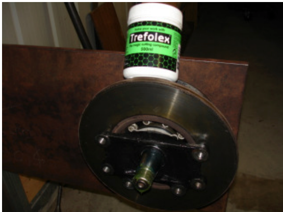
In production, the Factory supplied special grease for tightening the nut. In its absence my engineer friends suggested I use this product which beds in the threads and lubricates them.
