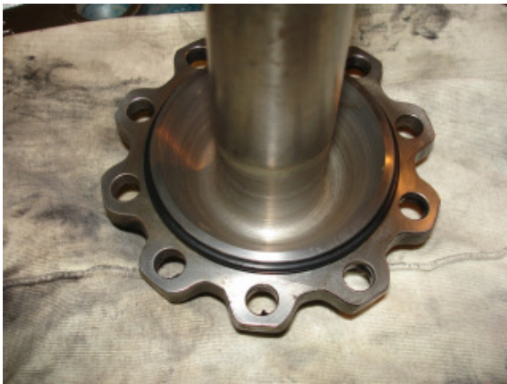
The drive shaft has a greased 'O' ring around its flange to keep out the crud. There is a small champher around the mouth of the axle to accommodate it.
