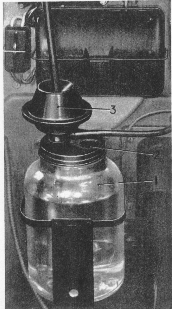
Fig. 49.—RESERVOIR AND PUMP.
