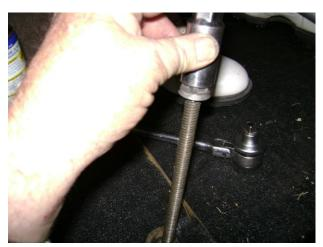
And if you are really thorough you will undo the nuts at the bottom of the lifting screw, screw the latter out, give it a good clean and grease-up and re-assemble.
