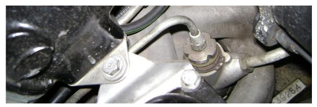
The outer casing can then be gently prised off, the 'O' rings replaced and the whole lot reassembled. The hazard?? This lies in the nipple in the supply line. It is easily cross threaded and with pumps on the fuel injected cars with an upward insertion fitting, this hazard is particularly popular! In these cases it is highly advisable to remove the bonnet so that you can work over the front of the grille.
