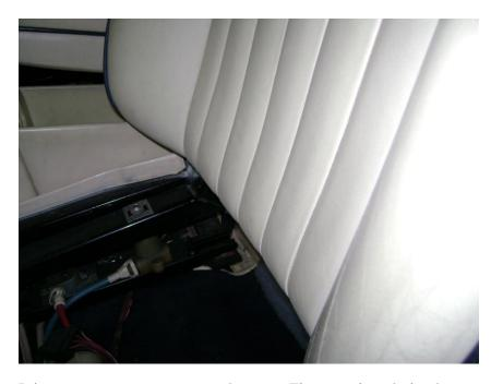
Here is the seat 'deflated. The 'bladder' sits under the padding immediately behind the pleating seen here. This padding and the rest of the leather cover is one unit that is stretched over a great hunk of moulded foam plastic and the seat frame!
