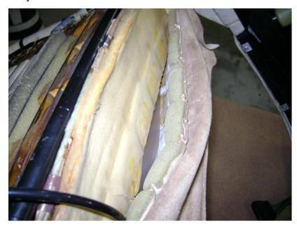
Here the pleated cover with padding has been pulled away from the foam block. It is the space between where the bladder needs to be placed.
