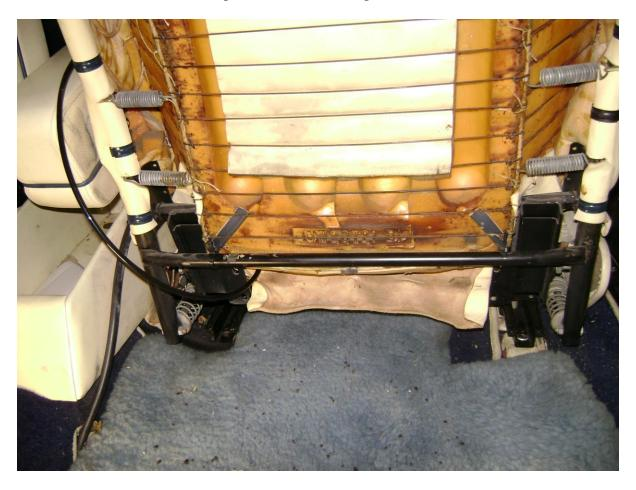
Here the bottom edge of the seat cover has been detached from the metal tube, bracing the bottom of the seat frame. The leather complete with clips simply pulls off, the clips are removed without tearing the leather or your fingers too much. Here can be seen the bulk of the squab – much foam with extra support from wires and springs etc! On this car on the driver's side which did not have the cross bracing, the anchor rod seen above had broken away at the side welds on both sides!
