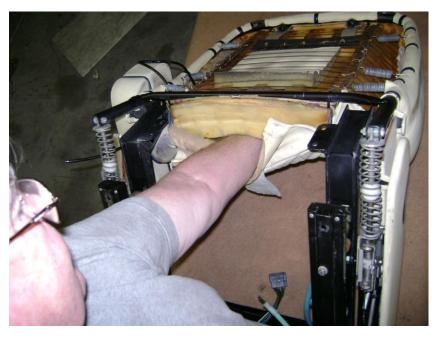
Thank you but I do not need captions for this picture. The seat in this case was removed while I worked out what to do and how. My probing hand with flexing arthritic fingers is wiggling its way into the bowels of the seat separating the cover from the cushion. This was the hardest part physically mainly because it hurt my fingers. The two items are not glued together but having been pressed together for the past 20
