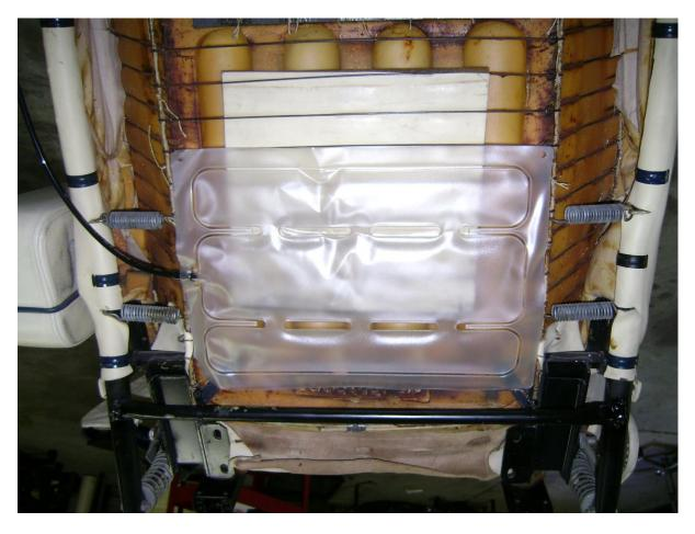
And here is the bladder available from any worthwhile auto upholsterer. The three inflatable sections are connected so that each can adjust to the shape of your back. The inflating tube is seen off to the left here.
