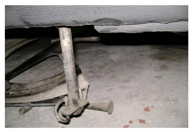
And here is the other bit of the modification. The small tube at lower left is intended to receive the wheel brace handle so that having lowered the wheel as far as possible the entire assembly can be lifted off the hook seen here at the bottom of the lowering tube. The spare wheel cradle has had added the holding bar seen poking to the right which in turn sits in the hook. And as seen below when you shoe the car with large mag wheels as on a Turbo, things are going to hang down a bit!
