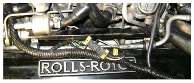
General advice is use only genuine pump kits as any others just do not seem to last. If you have the slightest doubt about the condition of the outer sleeve – that is the inside surfaces, have it re-sleeved by a good brake shop in stainless steel! The last picture shows the feed pipe for the front pump running along the top of the rocker cover. On this car the nipple thread on the feed pipe was damaged and the whole pipe had to be removed for repairs. Clearly a lot of mucking around!
