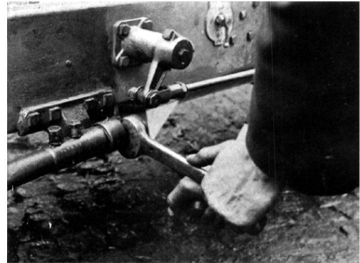
Fig. 55 ADJUSTMENTS TO BALL JOINTS ON RADIUS AND STEERING RODS, ETC.
