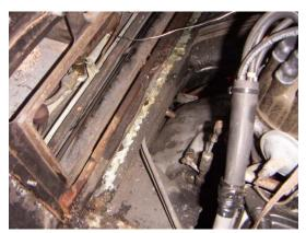
Another source of water is the condensate from the air conditioner evaporator. When the ice that forms on the fins melts it should run out the small pipe seen in the middle of the picture at left. This is the source of that embarrassing trickle that everyone puts up with when the car is parked on a hot day! If this tube blocks the water banks up and once more you have a flooding problem.
