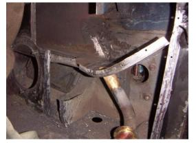
Unfortunately owners frequently cannot be bothered to keep the foam filter under the air intact grille intact, twigs bugs leaves etc get in and the drains block.
