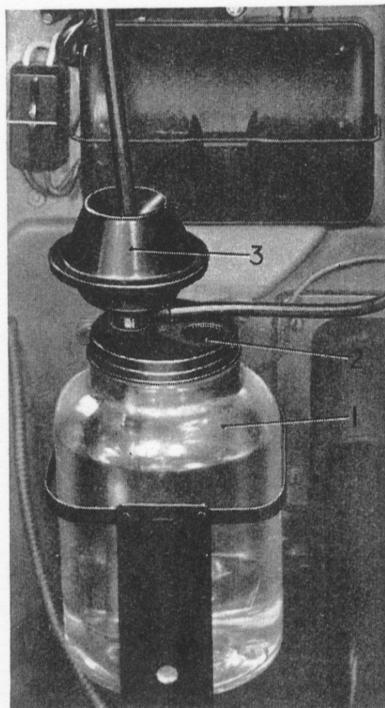
Fig. 49.—RESERVOIR AND PUMP.
