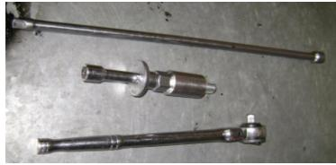
Nothing much new here except the centre collection. The very long extension is essential for the rear plugs on the 'B' bank of carburetted Shadows. With a little dexterity and patience the extension can be threaded down under the brake fluid reservoir and inserted into the plug tube spanner which is placed on the plug beforehand.
