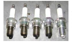
A typical example of fouled plugs through cold running and frequent starts and stops, The carbon build up simply shorts out the central electrode and the charge never gets to jump the gap at the and to create the spark. The end of the unglazed spark plug can just be seen on the new plug to the right.
