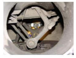
A bird's eye view of the suspension with the spring removed. The round object at the bottom is where the lower end of the shock absorber is housed and bolted in place. The clevis and rod disappearing to the right is the left hand caster rod that controls the fore and aft movement of that wheel.
