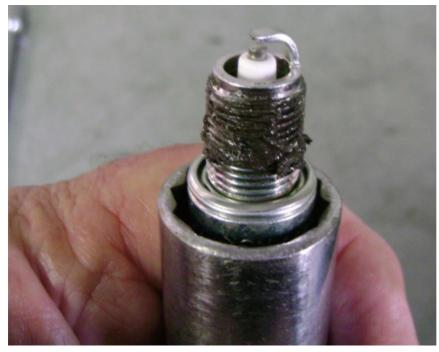
There are few hazards in plug changing. Apart from fitting the wrong plugs, avoid dropping them – they do not bounce. Note the anti-seize grease on the threads, something you should be using liberally around your car in the interests of preservation! Note also the metal sealing washer and its form. This crushes when you tighten the plug, a process you can feel in the spanner.
