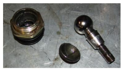
This is the lower joint opened for inspection cleaning and reassembly. The joint was quite loose. The adjustment for tightness is achieved by removing or adding shims between the upper cones seen at left and the body of the joint.
