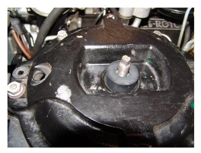
It remains to fit the top rubber bush and bolt down the top washer to the spacer.
