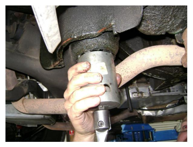
Here the locking ring on the top side has been removed and the bush is about to be screwed out of the sub-frame – note the anti-rust treatment via the leaking reservoirs. The tool in this case is a genuine factory item.
