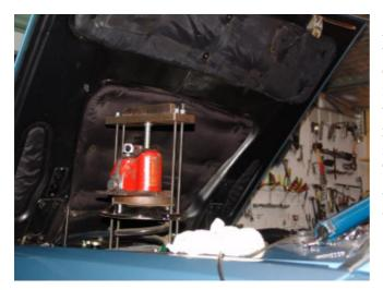
A heavy cross bar has been placed on the jack and connected to the body of the car with high tensile steel rods. The jack is fully extended and the cross piece tightened down on the jack. The remaining four bolts holding the top spring plate can now be safely removed. The jack is then slowly released allowing the spring to collapse the jack and release its tension.
