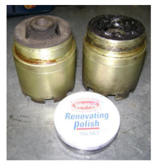
At left is a view of the two mounts inverted. The shoe polish tin is there to give a scale to the picture. The bushes are screwed into apertures at the rear of the sub-frame and locked by a screwed ring from the top side. The Factory method of removal is to disconnect everything and lift the body off the sub frame broadly speaking. My enthusiasm waned at this point so I hied me to my mentor and his hoist.
