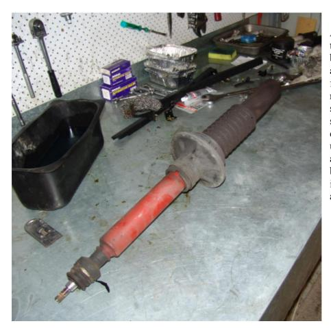
And here among all the mess on my bench is the shock absorbed plucked from the car after removal of the spring. The spring sits on the round collar seen halfway up the shock absorber. At the bottom of the latter is the joint we are aiming to tighten.
