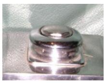
One picture saves a thousand words etc. Note the spring under the plug to aid withdrawal. Cars delivered new to Switzerland wore these caps and the lady was placed in the glove box. The hex key should be found in the tool kit and is a perfectly standard item!
