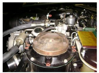
Here a thick steel mounting plate has been placed on top of the spring retaining plate with a felt cushion beneath. The latter is merely to prevent scratching of the paint on the plate beneath. The raised brackets on the mounting plate are to contain the particular jack used to release the spring tension. Note also the large hole in the
