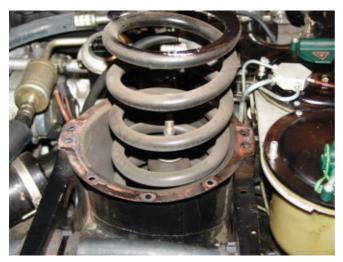
The removal apparatus has been taken away and the top plate lifted off with its damper washer. The top of the damper can be seen through the spring. It is important that the lower wishbones of the suspension are down as far as possible by removing the wheels. If this is not done the spring has that much further to emerge which cannot be accommodated with the jack.
