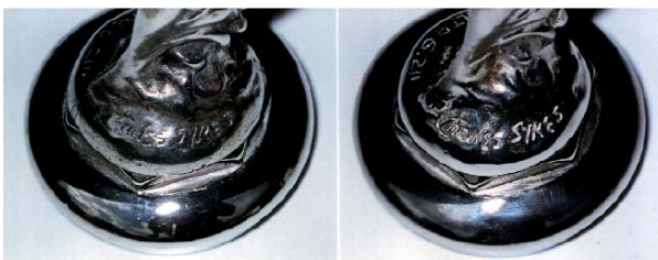
Left: an original Sykes mascot, somewhat pitted, but showing the appearance of inscriptions made in the wax pattern by a sharp point. Right: A reproduction mascot showing the appearance of lettering, after re-engraving with a fine dental bur. The writing is noticeably wider.
