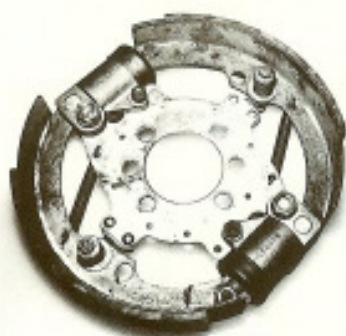
Figure 8: Front brake assembly after overhaul, but prior to refitting. Observe correct placement of bias springs—behind carrier plate. Figure 9: Brake shoes must be aligned square to the drum for maximum braking. Adjust the steady post: first screw it out part way, then adjust in with your square (made to size out of alloy) and a screwdriver. Figure 10: Brake drum with window cut out: this drum allows tightening of cylinder anchor bolts while brakes are on, thus centralized within drum. Handy here, it is a necessity for 4-shoe front brakes on Continentals. Be very careful when handling a brake drum. The cooling ribs are fragile and can be easily chipped—never hammer them.
