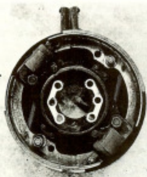
Figure 1: Complete front brake assembly, shoes and wheel cylinders, immediately after removal from car. When dismantling the front brakes, first undo the cylinder anchor bolts; then unbolt the whole carrier plate from the stub axle, starting inboard, so that the remaining components can be removed on the bench.
