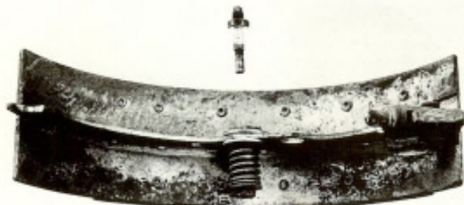
Figure 2: Front brake shoe and steady post which slips into shake back stop. Adjustment of post squares up shoes to drum. Figure 3: Shake back stop—exploded view. The shake back stop functions chiefly to hold brake shoes just at the interface when the brake pedal is released. It introduces friction into the system. Normally, such a device (in other makes of car) is built right into the shoe and is not adjustable, whereas Messrs. Rolls-Royce make theirs adjustable.
