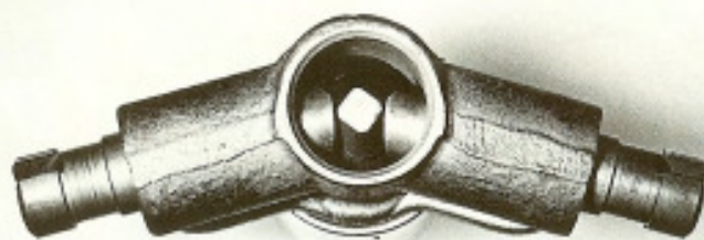
Figure 13: Rear brake adjuster unit plungers. They really are right and left handed. The notches fit locating pegs machined on the two bolts holding the adjuster to the backplate. Figure 14: Rear brake adjuster unit. If handed plungers are interchanged, the shoes will not contract enough to allow the drum to be refitted. When assembled correctly, turning the adjusting screw will produce an audible click.
