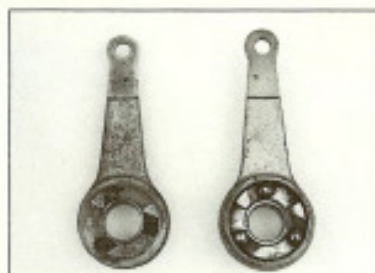
As the servo arms pivot during brake application, ball bearings on small ramps force the arms apart, engaging the servo which then assists in brake application. These bearings rarely wear. Use chassis grease to keep them from falling out during assembly.
