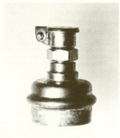
Figure 19: Rear brake equalizer and linkage. The pivot pin and bushes here were rusty, an indicator that the whole system, hydraulic and mechanical, requires attention. It is not enough to clean up this easily accessible unit and then stop. Figure 20: Author's modification: since there is no way to lubricate the pivot pin, I add an oil fitting to the cap over the pin. Then it's easy to put in a few drops of oil every time your car is serviced.
