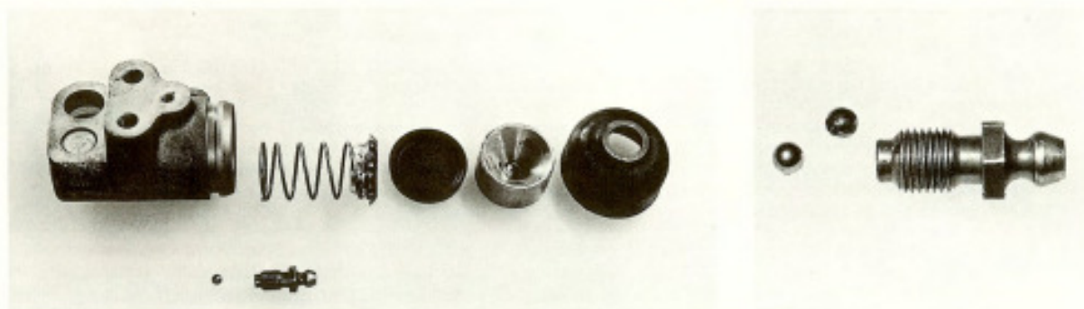
Figure 4: Front wheel cylinder, exploded view. The plungers in the cylinder should just pull out—with finger pressure only. If the plunger binds, carefully use compressed air to force the plunger out, say into a towel. If your system of compressed air is not sufficient to push the plunger out, use an hydraulic pump after making a fitting to the hydraulic line. Two hundred to 300 lbs. of hydraulic pressure should be enough for even the worst—or use a separate grease gun. The thread in the fluid pipe hole is the same as an ordinary 3/8 NF bolt. Be sure the plungers are the chromium plated type. A flawlessly smooth surface is what's wanted and needed here. Hone the wheel cylinders smoothish and clean. Surface finish and consistency are the goal for smooth working. Figure 5: Bleed screw with old and new steel balls. Discard the old ball. Do not lose the bleed screw balls in the cylinders. Remove the little ball from the cylinders first.
