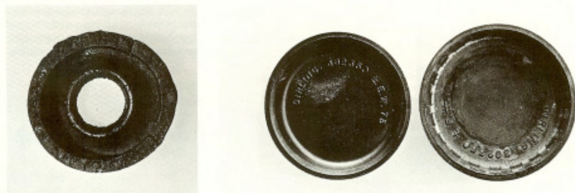
Figure 6: Water and dirt excluder for rear brake expander. Deterioration allows water and dirt into unit, which in turn corrode plunger and expander cylinder and damage rubber seals. Then brakes don't release. Figure 7: Rubber seals, front wheel cylinder. Left: new one; note sharp edges. Right: old and swollen, thereby binding brakes. Deterioration results from old age and soaking in brake fluid. You'll feel the difference between the old and new rubber parts. The old seals have expanded 3/16", are softer, and will bind in the cylinder. Replace all soft parts on overhaul. Don't argue. Just do it.
