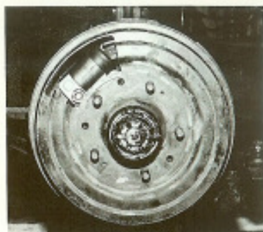
Figure 8: Front brake assembly after overhaul, but prior to refitting. Observe correct placement of bias springs—behind carrier plate. Figure 9: Brake shoes must be aligned square to the drum for maximum braking. Adjust the steady post: first screw it out part way, then adjust in with your square (made to size out of alloy) and a screwdriver. Figure 10: Brake drum with window cut out: this drum allows tightening of cylinder anchor bolts while brakes are on, thus centralized within drum. Handy here, it is a necessity for 4-shoe front brakes on Continentals. Be very careful when handling a brake drum. The cooling ribs are fragile and can be easily chipped—never hammer them.
