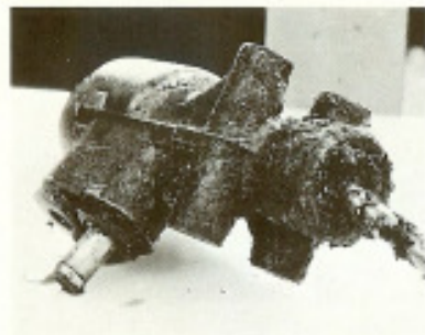
Figure 15: Master cylinder immediately on removal from car. Grit and muck indicate seepage and leakage—clearly time for overhaul. The muck is the result of a mixture of brake fluid and water attacking die-cast aluminum. Despite all the corrosion, these brakes worked, though they did not retract. You can inspect for corrosion without removal or disassembly: just look under the rubber covers. Figure 16: Master cylinder, exploded view. Notice corrosion on plunger at top right. Either fit replacement cylinders or bore and sleeve the old ones: cost considerations may dictate the method of repair.
