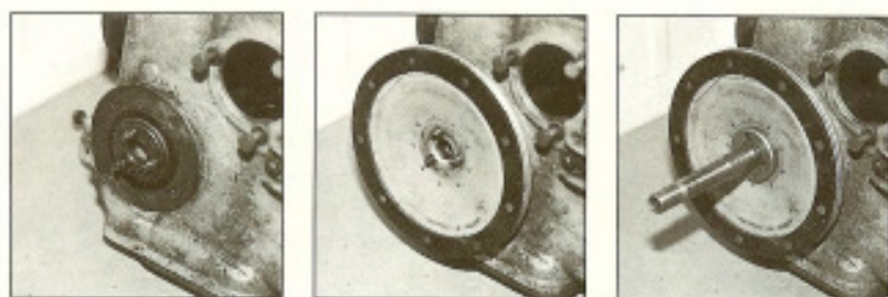
Left: Three prongs on the side of this early postwar manual gearbox help locate the servo mechanism. Removing the plate surrounding the prongs (remove 4 screws) exposes a replaceable seal. Center and right: The servo clutch plate and shaft fit onto the prongs after the whole servo unit is assembled. You must blindly twiddle the shaft to make it snap onto the prongs.
