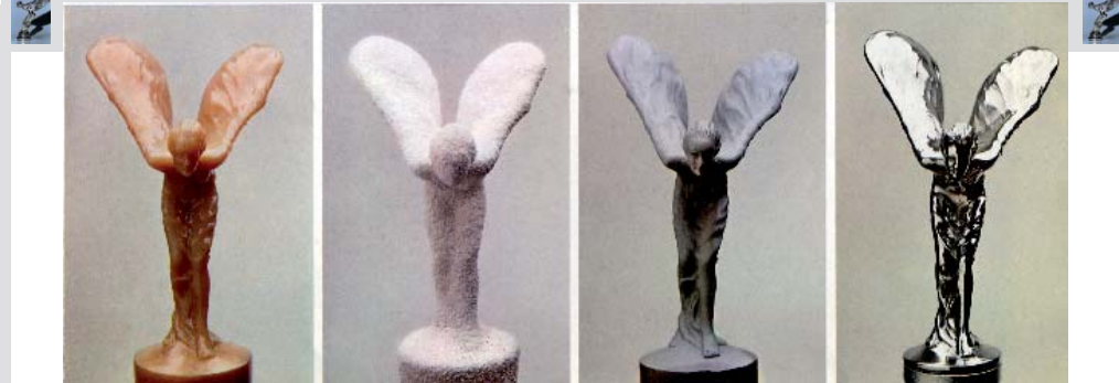
Post-WWII the Rolls-Royce company refined investment casting techniques for jet engine production. From left to right: an accurate wax pattern is made; it is sprayed with one of several refractory coatings; the sprayed pattern is surrounded by casting sand, the wax burnt out and replaced by molten metal and the solidified metal recovered; the metal casting, probably stainless steel, is polished.
