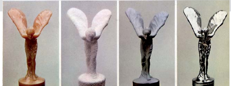
Post-WWII the Rolls-Royce company refined investment casting techniques for jet engine production. From left to right: an accurate wax pattern is made; it is sprayed with one of several refractory coatings; the sprayed pattern is surrounded by casting sand, the wax burnt out and replaced by molten metal and the solidified metal recovered; the metal casting, probably stainless steel, is polished.
