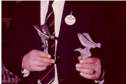
The Crewe employee, photographed here in 1960, is holding a semi-polished upright Silver Cloud casting, and an unfinished kneeling Silver Dawn or Silver Wraith unpolished casting. The first is probably stainless steel. The second appears to be stainless steel, but some were chromium-plated brass.
