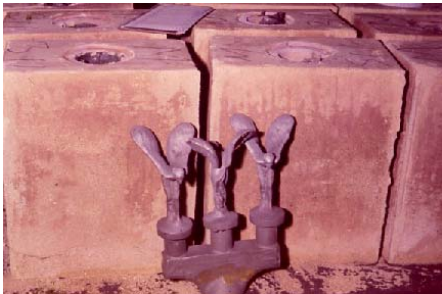
A casting of three wax patterns, mounted on a bar sprue. The original wax patterns were coated with a refractory, then surrounded by a block of casting sand to provide support. After wax burnout, molten metal was poured in to produce the castings shown here.
