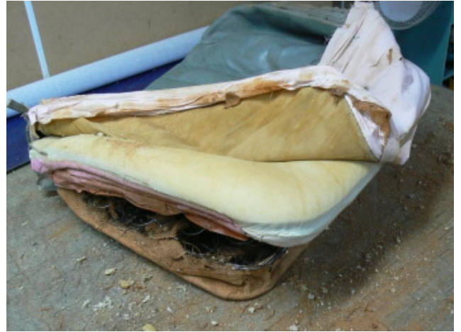
The cover almost off showing the moulded rubber horseshoe glued to all that is left of the original hessian.
