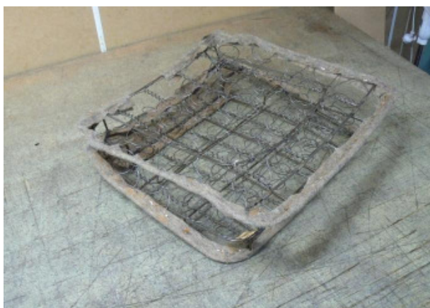
Stripped to the chassis with protective covers on the wearing bits, springing repaired where necessary.
