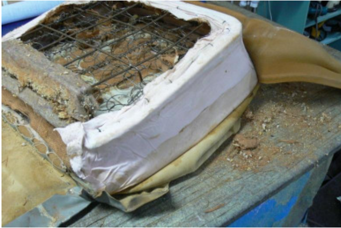
The calico wrapping had rotted and was about to disintegrate.
