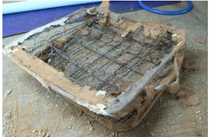
The 'hog ring' used to hold the leather cover in place. These are removed with the aid of side cutters and a strong wrist. The evidence of partial removal can be seen here!
