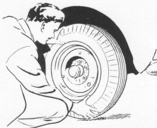
Fig. 30.—ENTERED STUD AT TOP.
