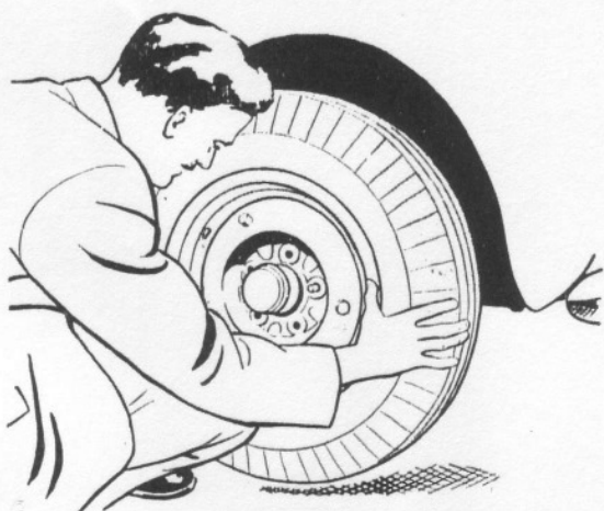
Fig. 29.—ROTATING FRONT WHEEL.
